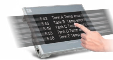
Scrolling the alarm messages
